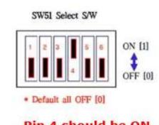
Pin 4 should be ON for using the VSR20D as Wiegand reader
